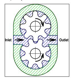
They can be used to put down long beads of adhesive or dispense encapsulation and moulding materials. Gear pumps are better suited to low viscosity materials they do not cause excessive wear on metal parts. If a metered shot is required, this can be done using a timer.
